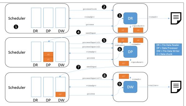
This example shows the data flow for a single scheduler loop. The basic scenario consists of reading data from a file, processing data and writing data into a file. The emphasis is put on the the data flow between the scheduler, its associated simulated boxes and their associated box algorithm (blue chip).
