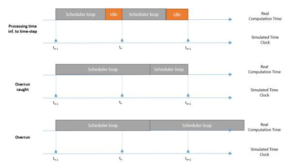
In the first case, real processing time is inferior to the fixed time step. During each time step, the system performs a scheduler loop. As the loop takes less time than the time step, the processor remains idle during the remainder of the time.
