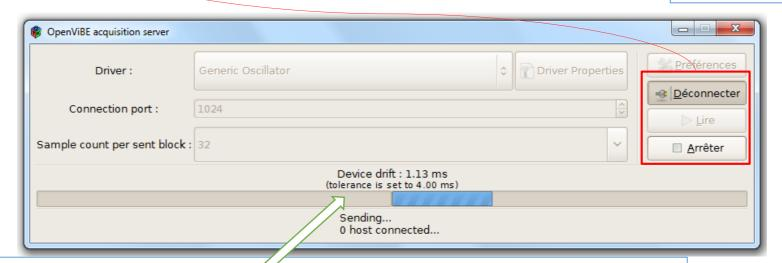
The acquisition reflects in realtime the device drift. The drift is the difference between the number of samples the driver sent to the acquistion server as compared to the number of samples it should have sent based on the elapsed time.
